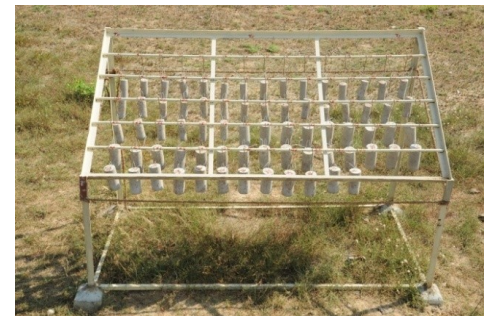
Fig.1. Specimens exposed at corrosion testing center, Mandapam
