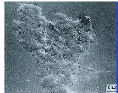
Fig. 4 Scanning electron micrograph showing crevice corrosion attack on 304 SS specimen after the biofilm was removed
